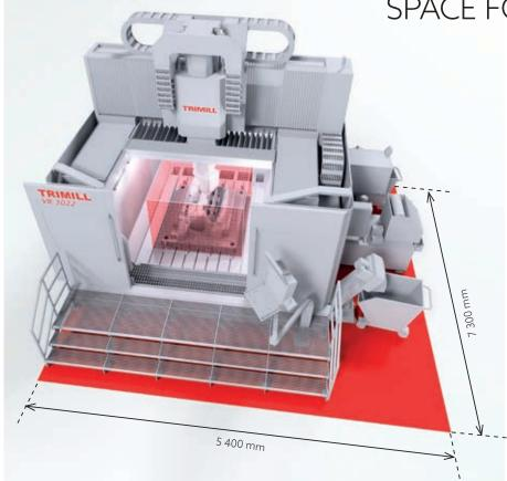
A significant competitive advantage is the minimum installation area of the machine (only 39 m²) compared to the maximum machineable part size (up to 7.6 m²).
