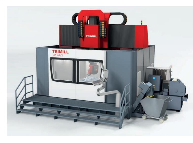
The TRIMILL VR line of 5-axis gantry machines is specially developed for high-speed semi-finishing and finishing milling. The key technical parameters are the high speed of working feeds (60,000 mm/min.) and acceleration (max.  $6 \text{ m/s}^2$ ), which are achieved by using linear motors and a weight-optimized crossbeam.
